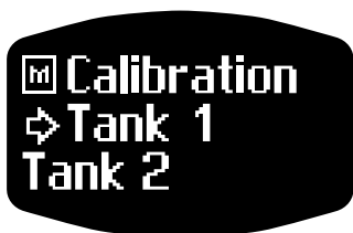
Figure 1-49: Selecting a Fuel Tank to Configure.
